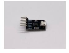
2. Connect the 6 pins cable that came with the Flight Controller to the microUSB board according to the following table (there's one unused GND pin on the board).
