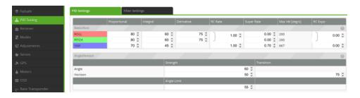
Fig. 121 GUI tab in CleanFlight to set the PID values (with recommended starter
