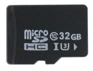
The micro SD card stores the operating system on the Raspberry Pi, as well as all the software needed for autonomous flight.
