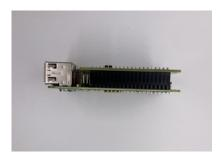
Fig. 47 Raspberry Pi Hat inserted into Raspberry Pi pins
