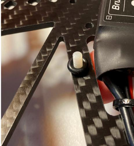
3. Screw the nuts on the bolts from the bottom side.
