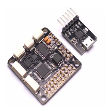
Fig. 78 OSD version Flight Controller
