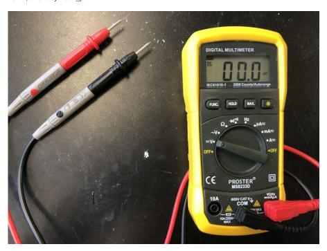
$\textit{Fig. 5} \ \text{Switch the Dial to the DC Voltage Test Function}$
