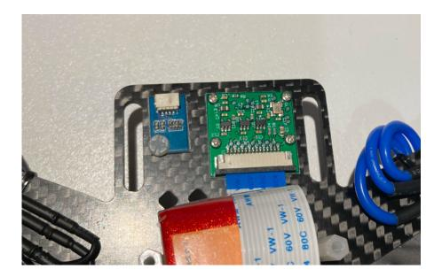
$\textit{Fig. 98} \ \text{Camera (and ToF sensor) attached to the front of the frame}$
