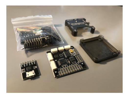
Fig. 72 OSD Flight Controller
