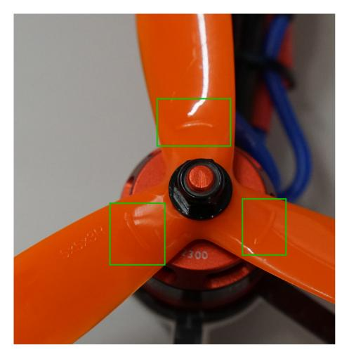
Fig. 109 Arrows on the propellers indicating spin direction
