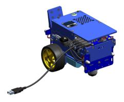
Once your Duckiebot is fully charged, you can press the button of the battery on the side to power it up (do this ONLY if a flashed SD card has been inserted).
