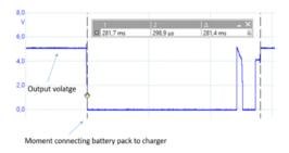
Fig. 66 The Duckie Power Bank output voltage drops when plugging in and removing the charger.
