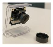
Fig. 15 The camera on its mount.
