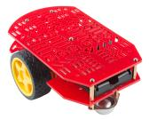
Fig. 7 The "Magician" chassis was very popular. It is used in DB17 through DB19 Duckiebot models.
