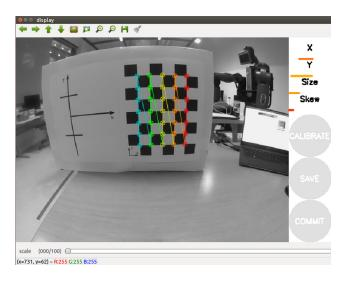
Fig. 50 Intrinsic camera calibration tool
