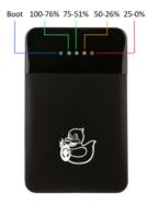
Fig. 60 LEDs indicate the state of charge of the Duckiebattery.
