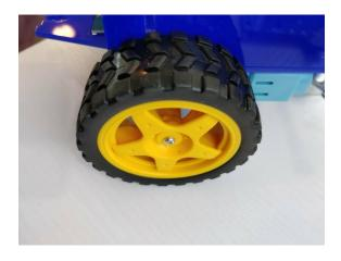
Fig. 36 Screws will keep the wheels in place. Do not tighten too hard!
